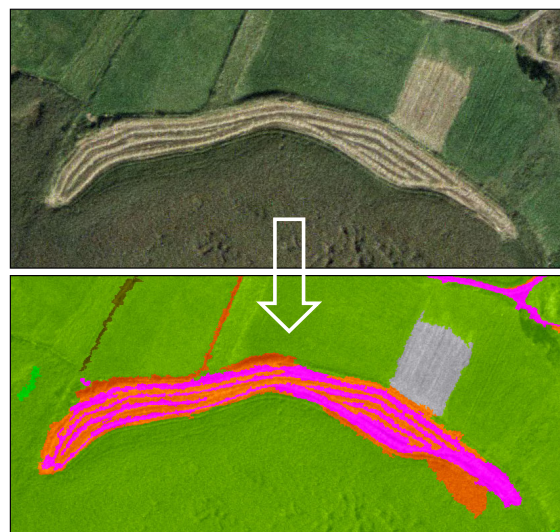
Figure 6. Example of confusion between a mowed reed plot and a concatenation of connected linear elements likely to form part of the trail network
